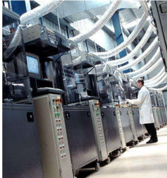
CFCL-Fuel cell test station
