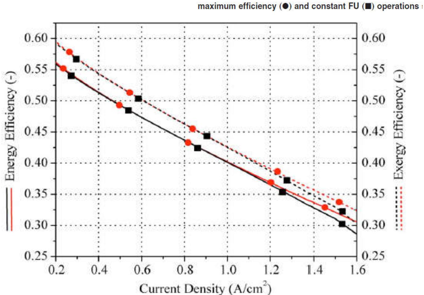
constant FU operation of the fuel cell at a particular value of FU can closely approximate the maximum efficiency operation of the fuel cell
